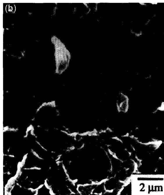
Figure 5 SEM scans of fatigue fracture surface of a 10/90 blend of SPS ionomer (2.65 mol%) and PS: (a) entire fracture surface; (b) high magnification scan showing two-phase nature of blend
