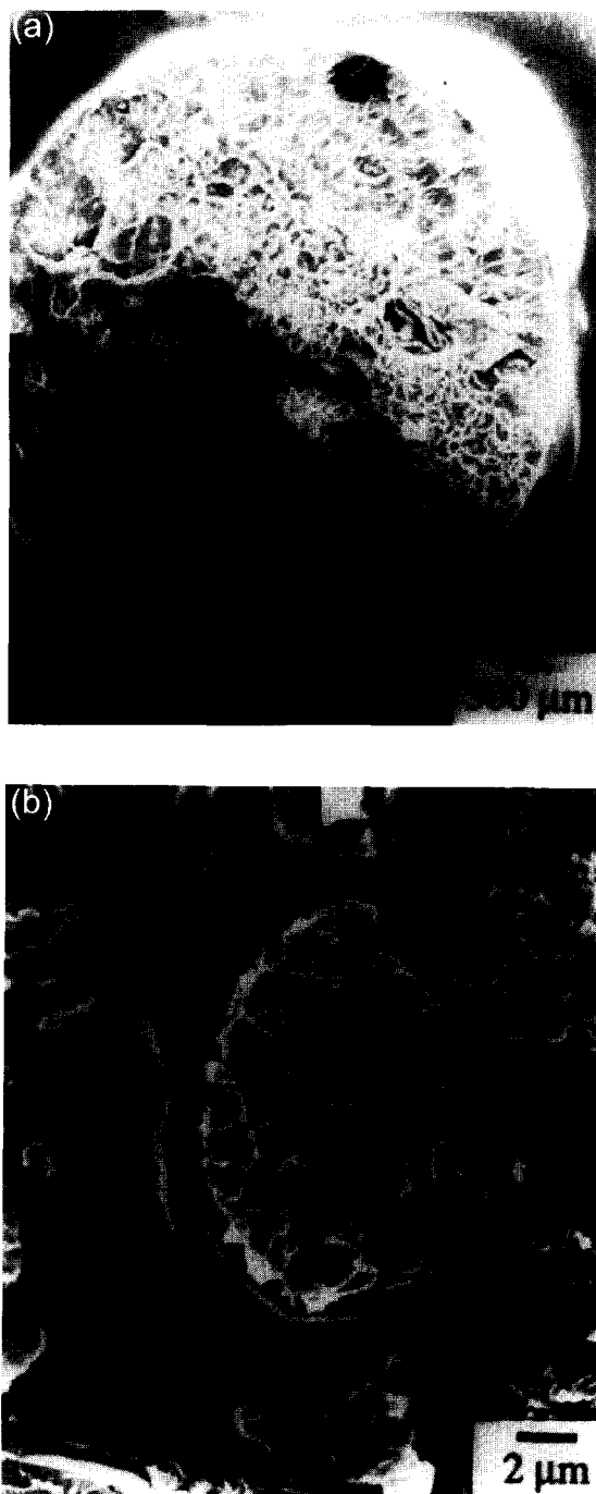
Figure 8 SEM scans of fatigue fracture surface of a 10/90 blend of SPS ionomer (7.48 mol%) and PS: (a) entire fracture surface; (b) high magnification scan showing a large ionomer particle
